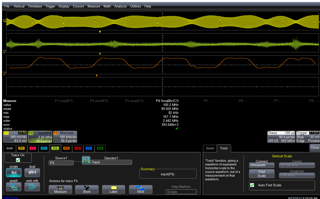
Figure 6: Using the track of the frequency@level parameter and a low pass filter to demodulate C1
