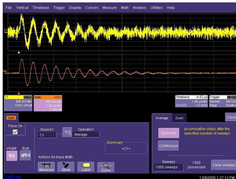
Figure 1a: The upper trace is the raw samples from the ADC. The lower trace is 1000 averages. The noise (from the signal and from the acquisition process) are greatly reduced by averaging.
