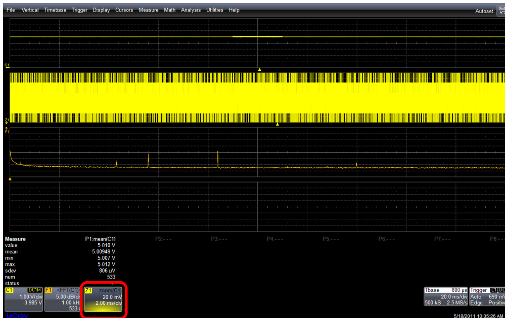
Figure 3a: The flat line in the upper trace is from a DC power supply. The middle trace is a zoom, showing 8 divisions of noise at 20 mV/div (red box). The lower trace is an FFT.
