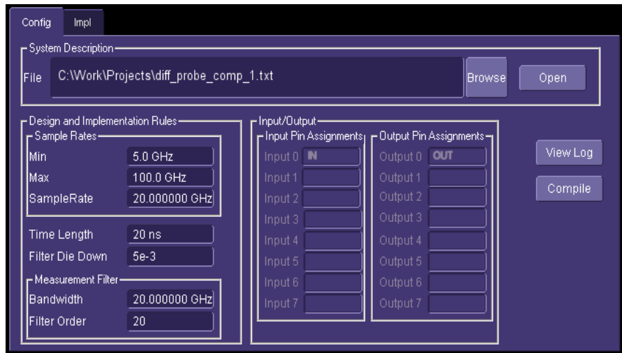
Figure 5: The setup for the Virtual Probe math function.
