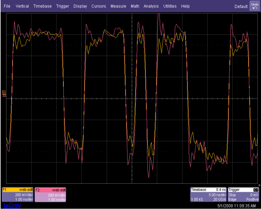
Figure 7: A comparison of the “loaded” (trace F1) and “unloaded” (trace F2) responses of an 11 GHz probe using a 13 GHz Scope
