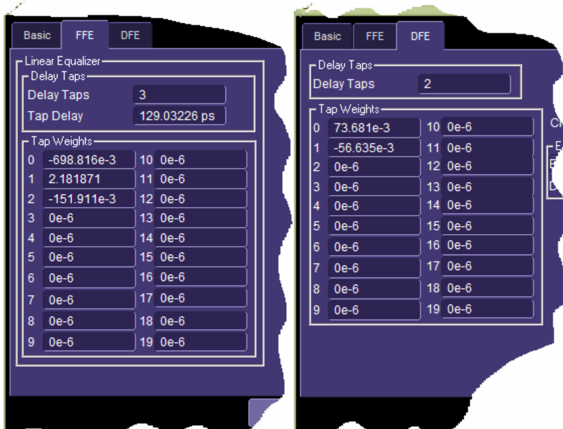
Figure 9 – Equalized Receiver Dialog Showing Manual Filter Tap Settings
