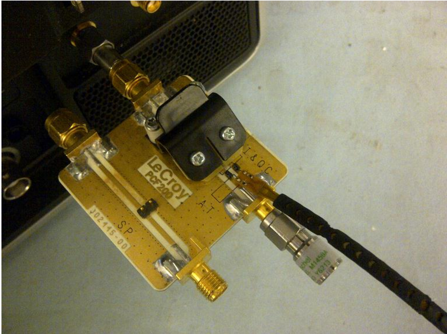
Figure 1: Recommended Configuration for Deskewing: PCF-200 terminates with 50-ohm coaxial termination
